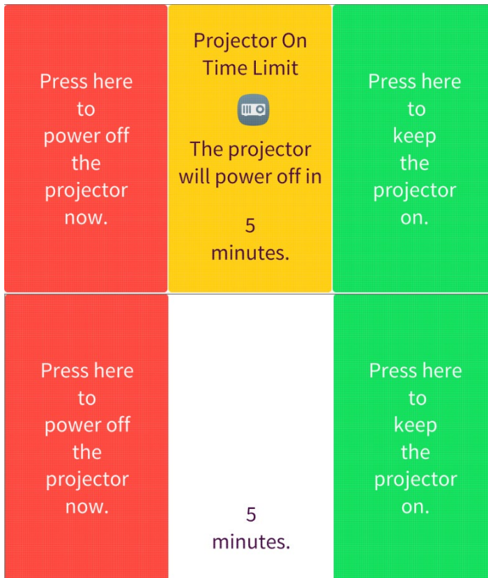
Figure 28 Projector Auto-Off Sequence with Center Panel Flash
